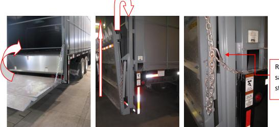
Reattach limit safety chain in stowed position.
