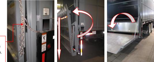
Unlatch Safety limit chain from stowed position.
